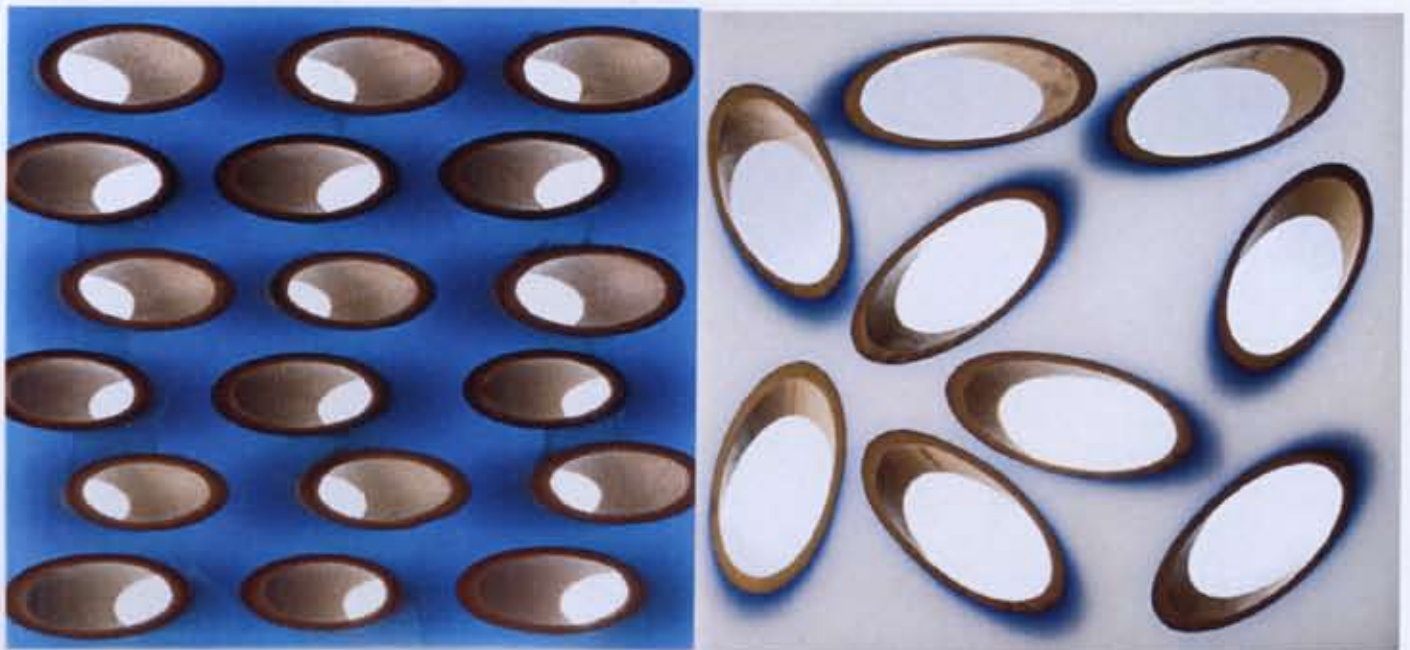
Figure 4.15: New material by Yvonne Laurysen and Erik Mantel (Lama Concept) made from the stem Main processing technologies used: sawing and casting
